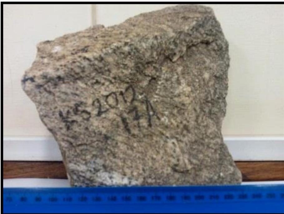
Fig 5.4.2. Gneiss exhibits folded leucocratic veins in hand sample. The leucocratic veins consists of coarse-grained quartz, plagioclase and microcline.
