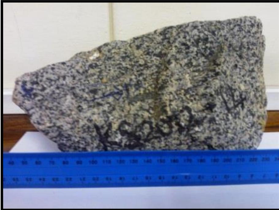
Fig. 5.4.1. Foliated coarse-grained granodiorite. The rock consists of hornblende, biotite, plagioclase, microcline, quartz, epidote, chlorite and Fe-Ti oxide.
